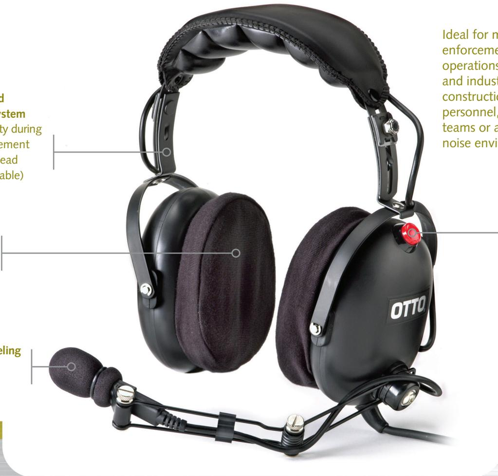
OTTO **ClearTrak heavy duty headsets** are IS/ATEX certified and offer a certified noise reduction rating (NRR) of 24dB. Fitting snugly to the head, the headset can be worn comfortably under a helmet. The push-to-talk switch is positioned on the ear cup for added convenience. ClearTrak offers superior intelligibility and the additional hearing protection necessary for consistent, clear communication.
